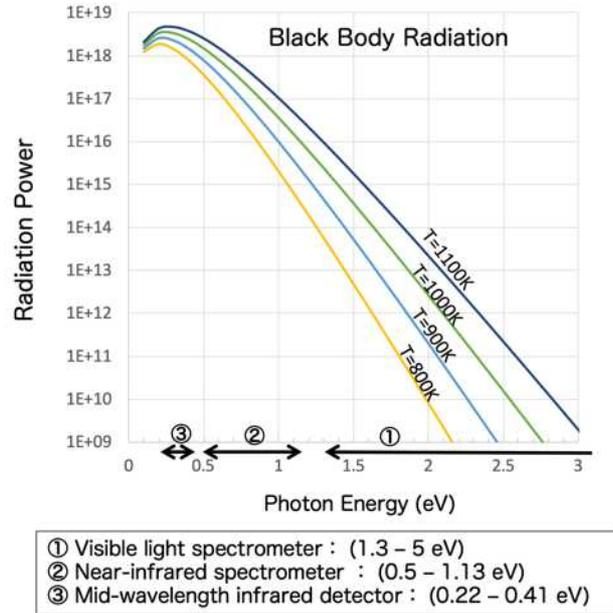
Fig.10 Extended spectra; from Visible light to infrared.
