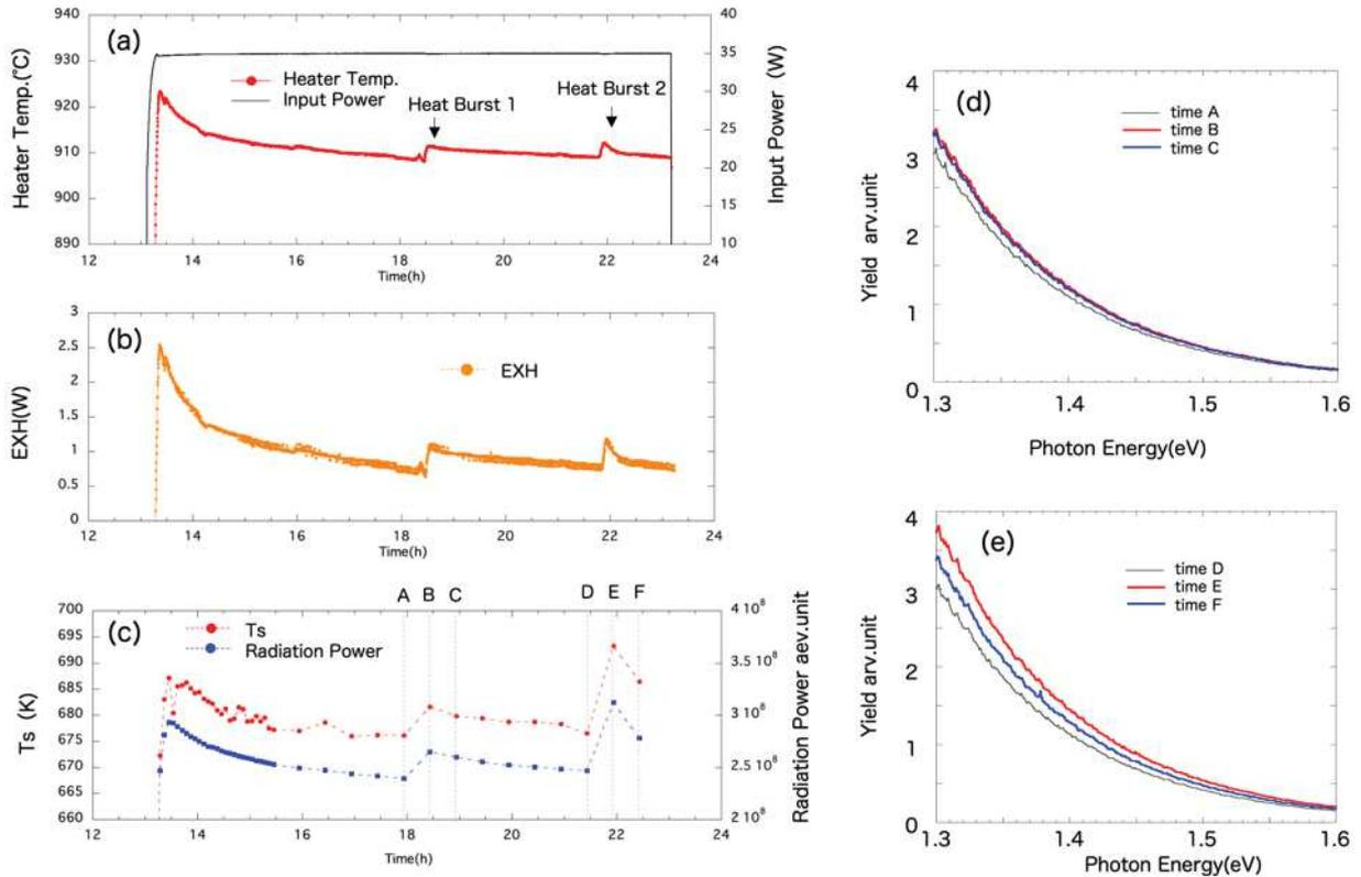
Fig. 9 Simultaneously detection of Heat Burst by Radiation of spectrometer Looking at the Surface of the Multilayer Thin Film and a Thermocouple Located in the center of Heater. (a)Heater Temperature and Input Power, (b)Excess Heat, (c) Surface temperature and Radiation Power by Spectrometer, (d)Radiation Spectrum of 1<sup>st</sup> Heat Burst, (e) Radiation Spectrum of 2<sup>nd</sup> Heat Burst.
