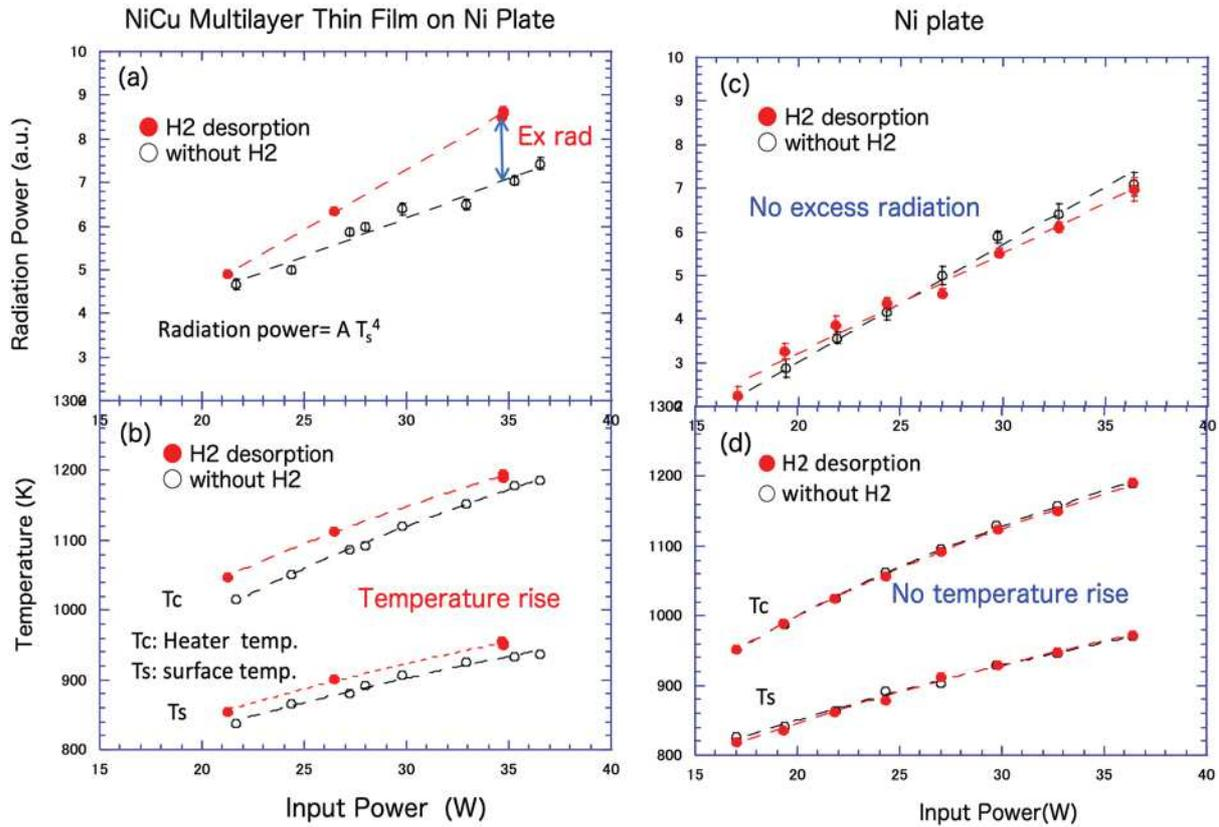
Fig. 8. Comparison of emitted radiations between NiCu Multilayer Thin Film on Ni Plate and Ni Plate. (a) Radiation Power and (b) Temperature of experiment using NiCu Multilayer Thin Film (c) Radiation Power and (d) Temperature of experiment using Ni Plate.
