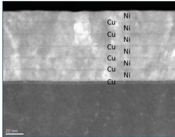
Fig. 5 Scanning Transmission Electron Microscope (STEM) Image of Cu-Ni Multilayer Thin Film.
