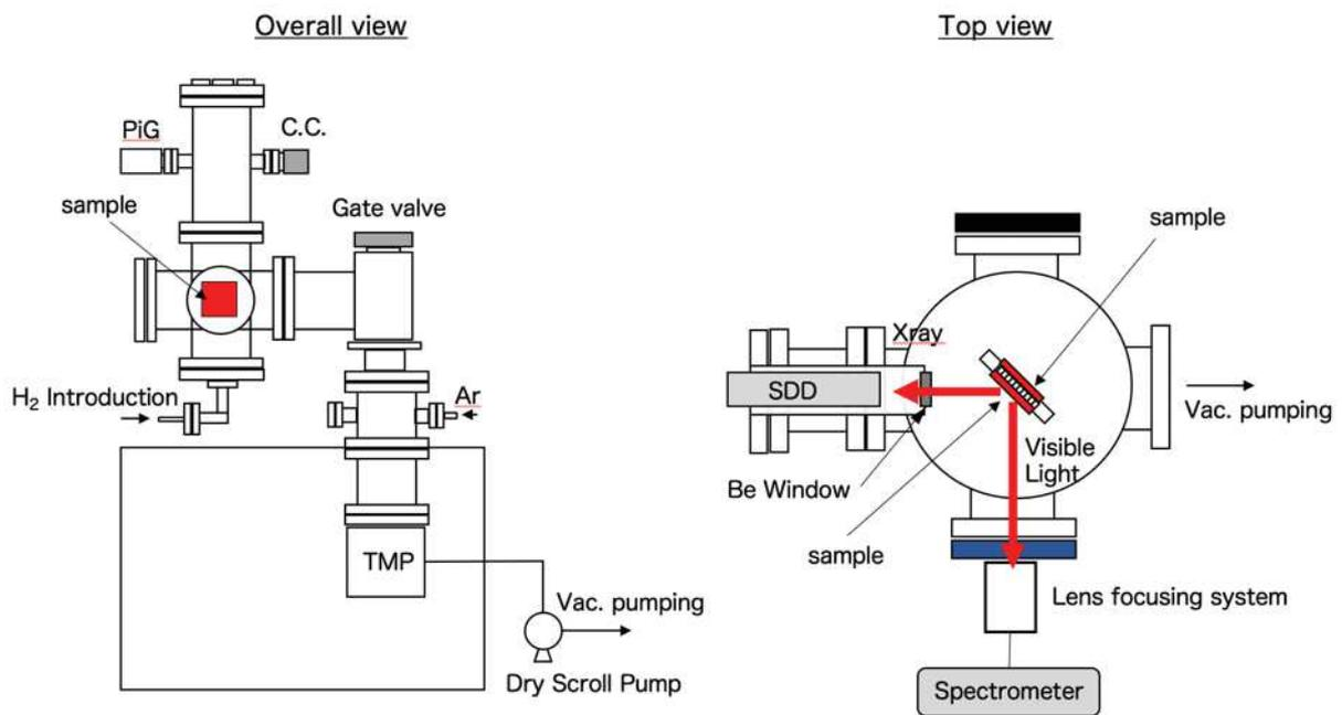
Fig.4 Schematic of Experimental apparatus.
