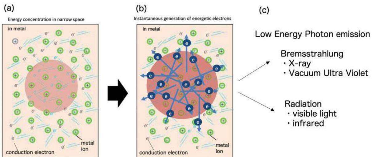
Fig.3 Schematic of energy distribution to electrons when energy is generated locally. (a)Energy concentration in narrow space, such as a nuclear reaction, (b)Instantaneous generation of energetic electrons, (c)Low Energy Photon Emission due to energetic electrons
