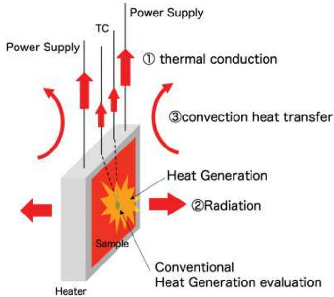
Fig.2 Heat transfer path when a heat generation phenomenon occurs.
