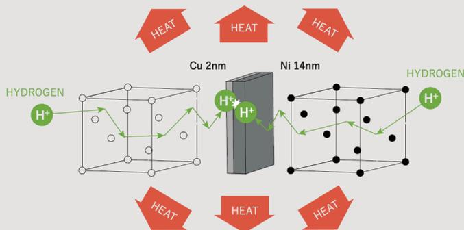
Unlike plasma-based fusion, which requires confinement of hydrogen isotopes at over 100 million degrees Celsius, Clean Planet's Quantum Hydrogen Energy (QHe) operates within a solid metal lattice at temperatures below 900 °C. Hydrogen atoms penetrate the nanostructured lattice, where quantum effects within specific defects appear to trigger a form of nuclear-level heat release. The process emits no neutrons, gamma rays, or radioactive by-products, making it safe for direct industrial deployment.
